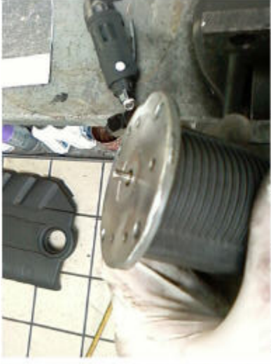
You can now depress plunger and notice one hell of a difference. at this point you will have to clean the body of the valve in some form of cleaner.
