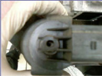
drill a 3mm hole in top of valve as shown
