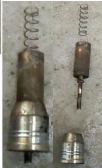
What you should have when you have tapped out insides of solenoid now you will see the real cause for the egr complaint these parts will be corroded and cause sticking, believe it or not its not the soot that jams the valve but this corrosion
