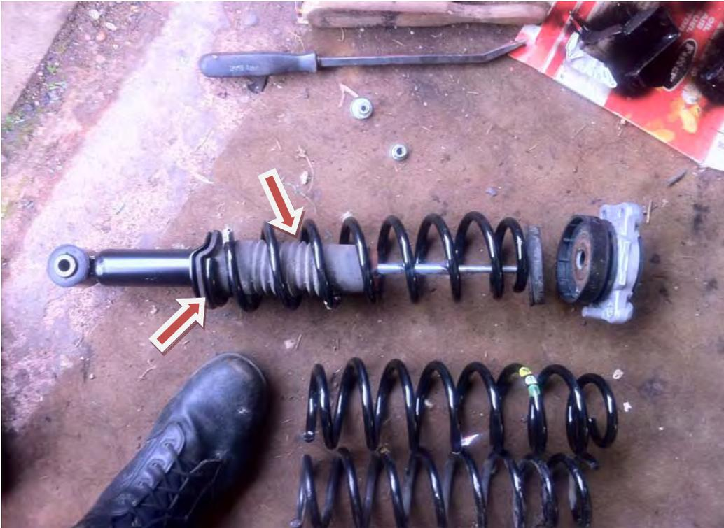
14. Well that's half the job done or a quarter if you are doing both sides. Remember to swap over the rubber from the bottom of the strut to your new one and gaiter from the centre.
