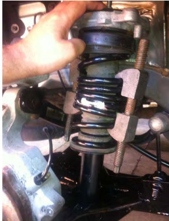
12. Now remove the bottom pin, the 21mm head one and lift out the suspension strut.
