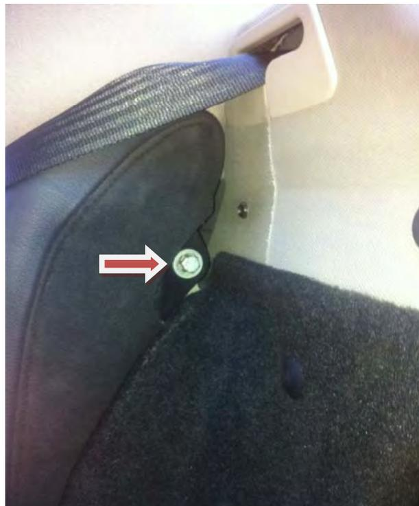
3. Once the bolster is free to move you need to release the two plastic pegs which hold the black carpet trim in position.
