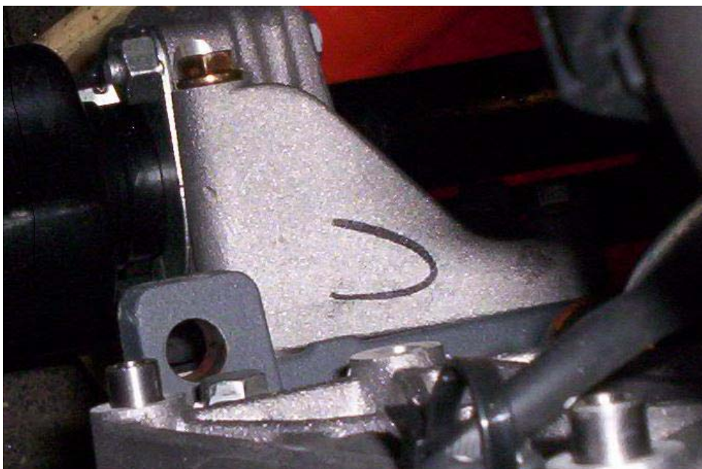
Right axle shaft support for 1.3 Multijet 90 HP version
