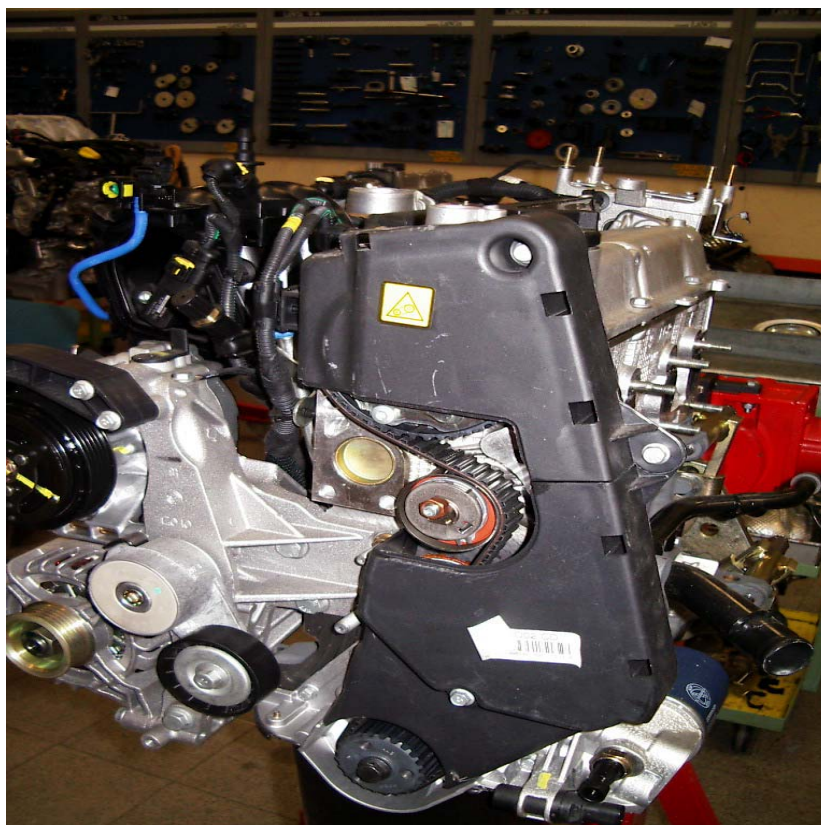
Timing belt upper and lower protection
