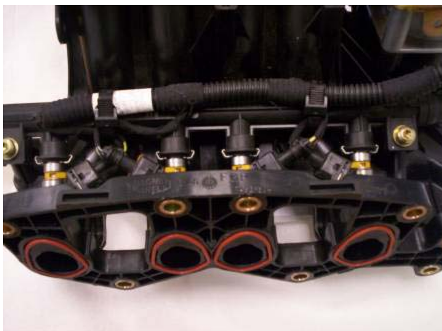
Injector housing on the intake pipe
