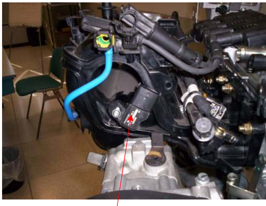
Sucked air pressure and temperature sensor
