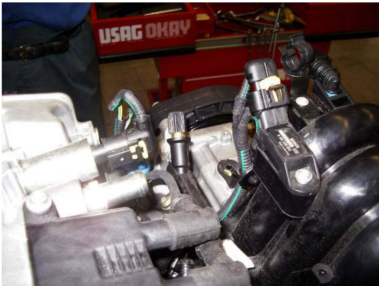
Atmospheric pressure sensor position
