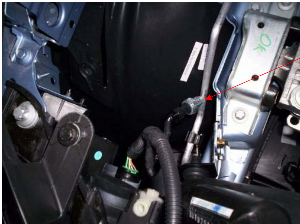
1: A/C linear pressure sensor (placed on the high-pressure duct)
