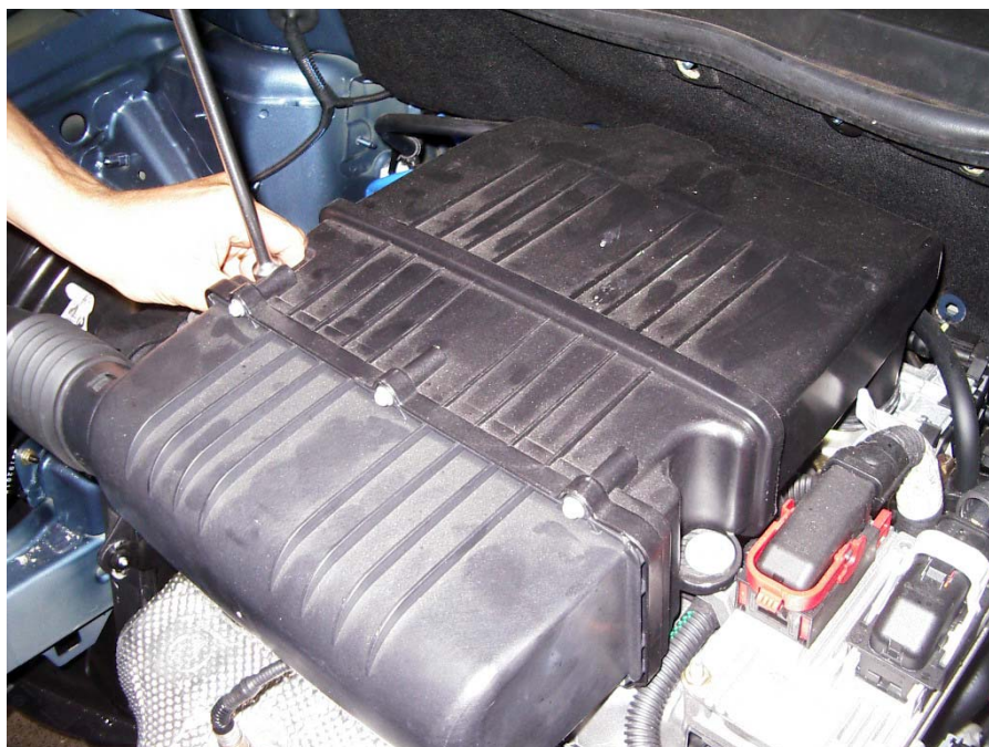
Air filter fastening screws
