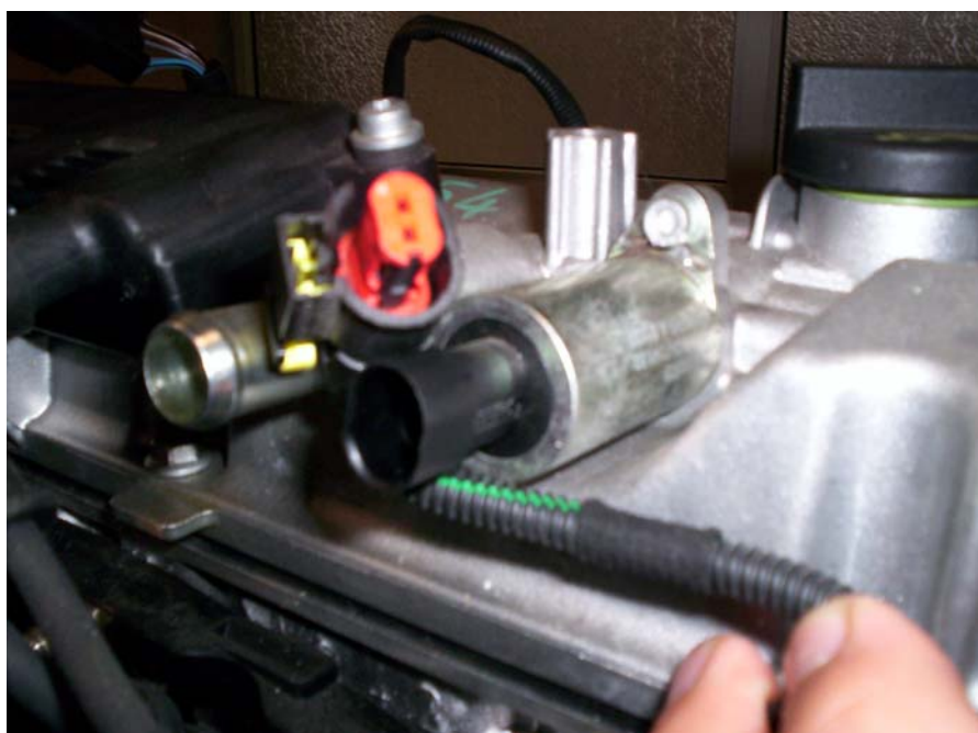
Phase variator control electromagnet with its respective connection
