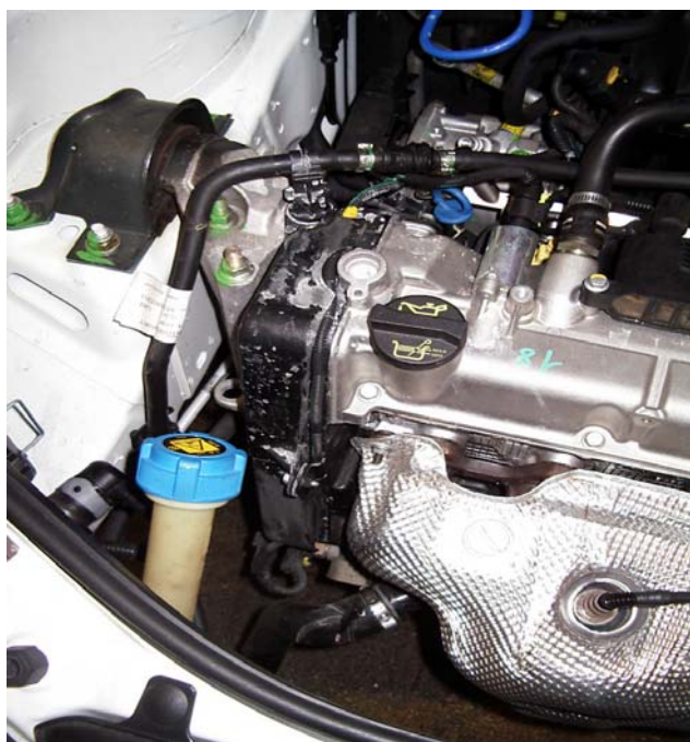
Power unit support (valve gear side)
