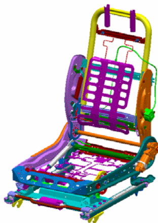
Electrically-adjustable front seat structure
