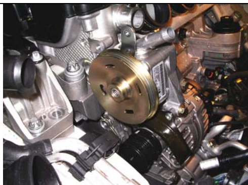
Power steering pump location
