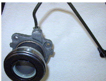
Annular cylinder fitted on M32 transmission clutch bell.
